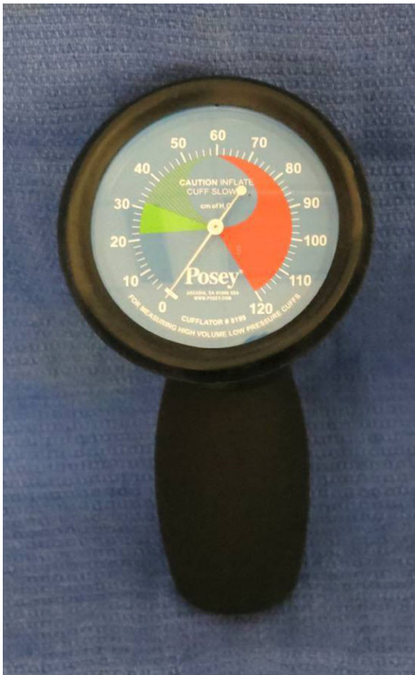
Figure 3 Commercially available hand-held manometer for inflation and measurement of intracuff pressure (Posey Cufflator Endotracheal Tube Inflator and Manometer™; JT Posey Company, Arcadia, CA, USA).
